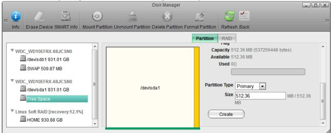
Assuming that the capacity of your new drive is identical to the existing drive, we suggest creating a SWAP partition. To do so, select the Free Space, open the Partition tab and click Create. The partition type and size can be left at default.
