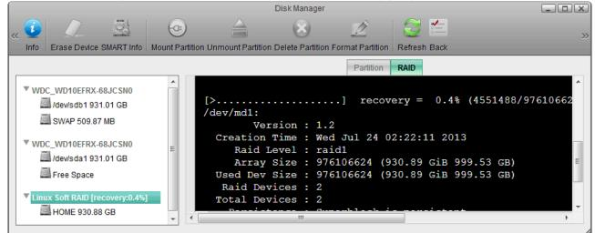
6. Depending on the capacity of the new drive, you will have some additional free space. If the capacity is identical to the existing drive, the remaining space can be used for SWAP. If the capacity is larger, you can create an additional partition for extra storage. Either way, to make use of this free space, you will have to manually create a partition, format and mount it.
