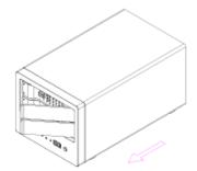
Install the hard drive, making sure the connector is facing the open side of the bracket. Slide the tray back into the enclosure and push the handle lightly into place.
