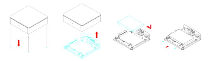
Replace the top enclosure. Fasten the screws on the bottom of the case, place the rubber feet over the screws and stick them on the casing to cover the screws.
